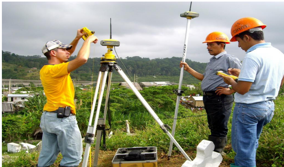
Figure 2. GPS equipment with RTK differential GNSS technique
