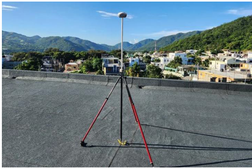
Figure 6. GNSS Receiver at Base Point on the roof of the Altagracia Brito School
